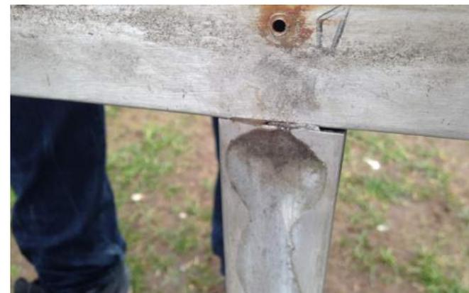
I'm pretty sure that these bars are actually welded , not folded sheet metal like I originally assumed. They have polished the weld lines off impressively on the front faces of the frame if this is the case.
